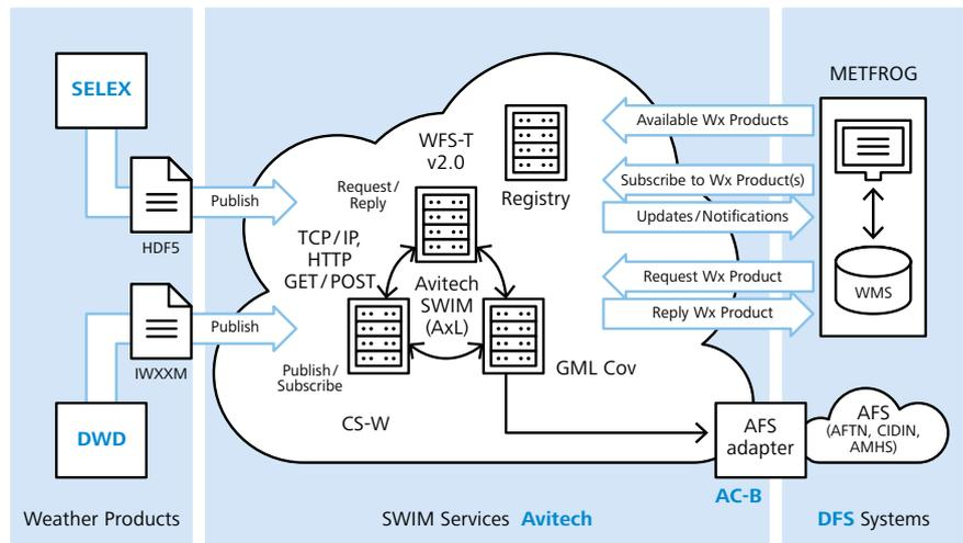
**WeAC** provides geo-referenced products using highly sophisticated sensor technology and data fusion algorithms. The Ground Weather Monitoring System supplied by Selex ES and ITWS – Integrated Terminal Weather System supplied by DWD are ensuring the provision of cutting-edge meteorological products for the ATM user.
